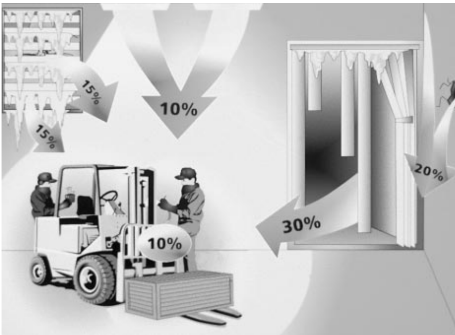
Figure 3 Heat loads on a cold store as a percentage of the total heat load
