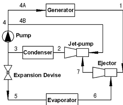
Fig. 3. A new ejector refrigeration system.
