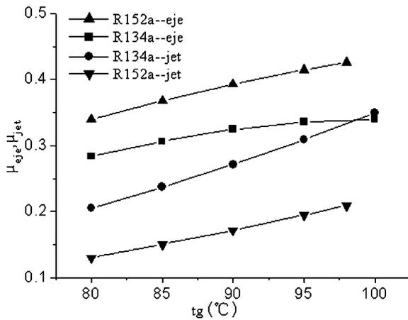
Fig. 5. Variation of entrainment ratio with generating temperature.
