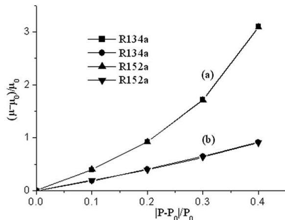
Fig. 4. Variation of relative change rate of ejector entrainment ratio with secondary pressure or backpressure.
