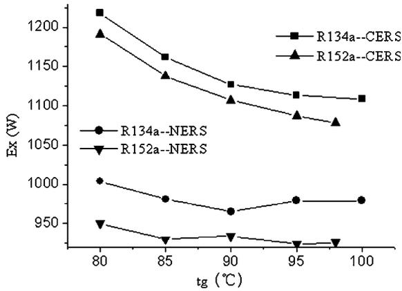
Fig. 9. Variation of input exergy with generator temperature.
