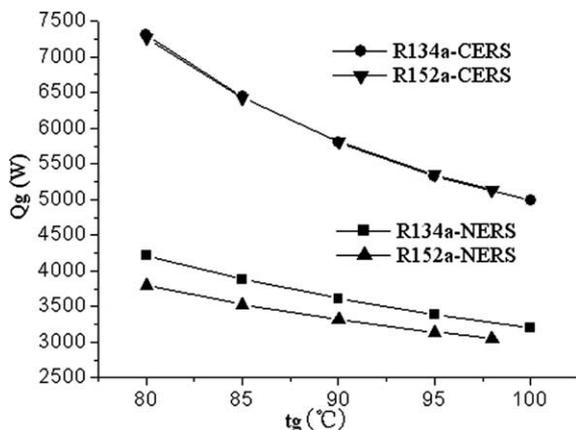
Fig. 6. Variation of generator's heat load with generating temperature.
