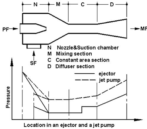
Fig. 2. The variation of pressure in ejector or jet pump.
