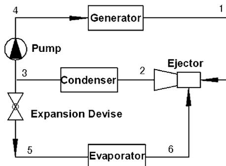
Fig. 1. A conventional ejector refrigeration system.
