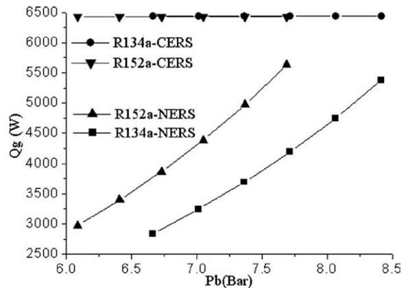
Fig. 11. Variation of generator's heat load with backpressure.
