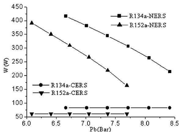
Fig. 12. Variation of pump work with backpressure.
