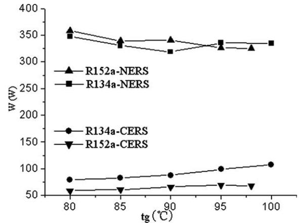
Fig. 7. Variation of pump work with generating temperature.
