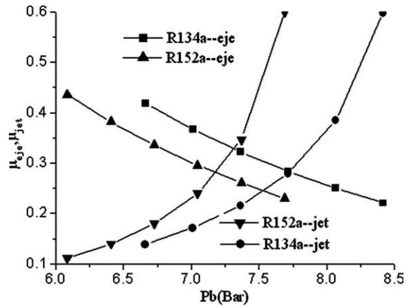
Fig. 10. Variation of entrainment ratio with backpressure.
