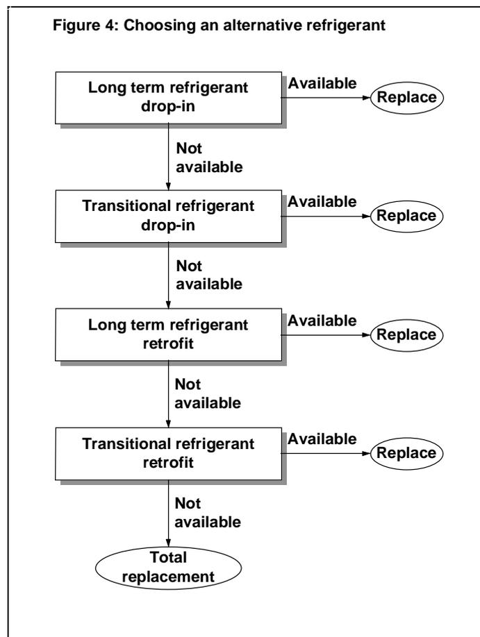
Applying the logic of Figure 4 to the table of R12 alternatives in Figure 5a gives the following results (similar logic can be applied to the table of R502 alternatives in Figure 5b):
