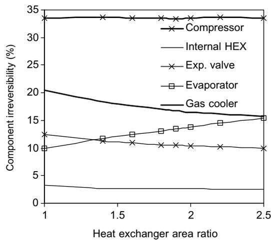
Fig. 3. Variation of component irreversibility with heat exchanger area ratio.
