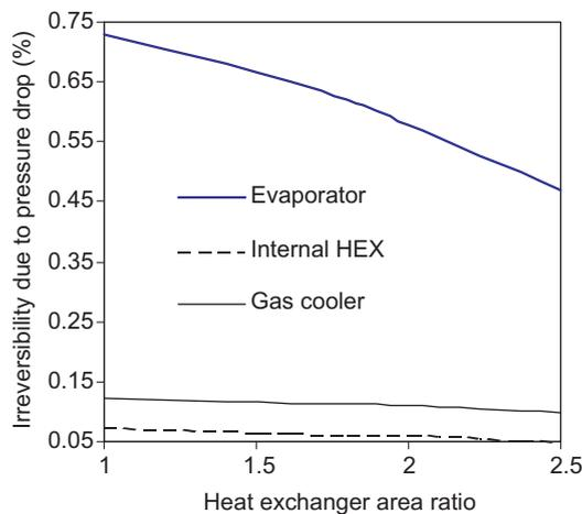
Fig. 4. Influence of heat exchanger area ratio on irreversibility due to pressure drop.
