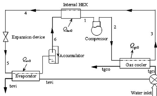
Fig. 1. Schematic layout of a transcritical carbon dioxide heat pump system.
