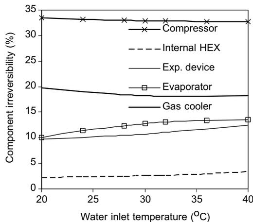
Fig. 6. Variation of component irreversibility with water inlet temperature.
