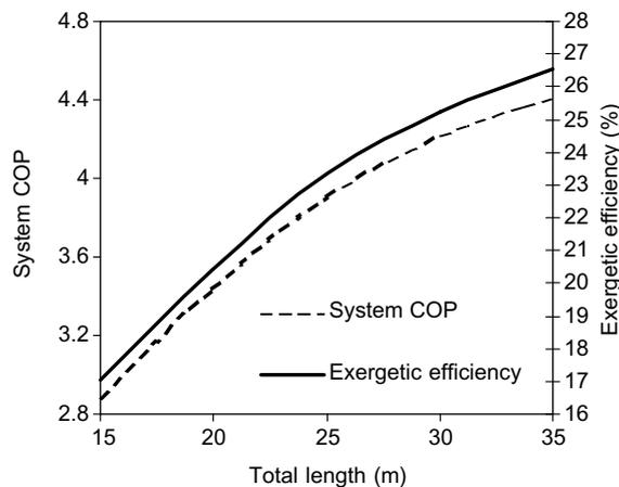
Fig. 10. System performance with varying total heat exchanger length.
