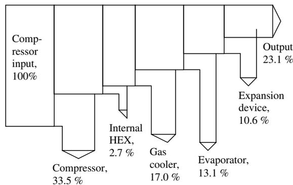
Fig. 8. Exergy flow (Grassmann) diagram at mean operating condition.
