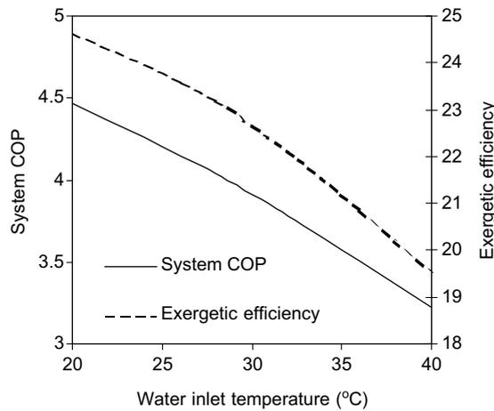
Fig. 5. System performance with varying water inlet temperature.
