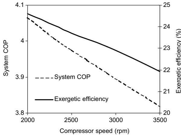
Fig. 7. Effect of compressor speed on system performance.
