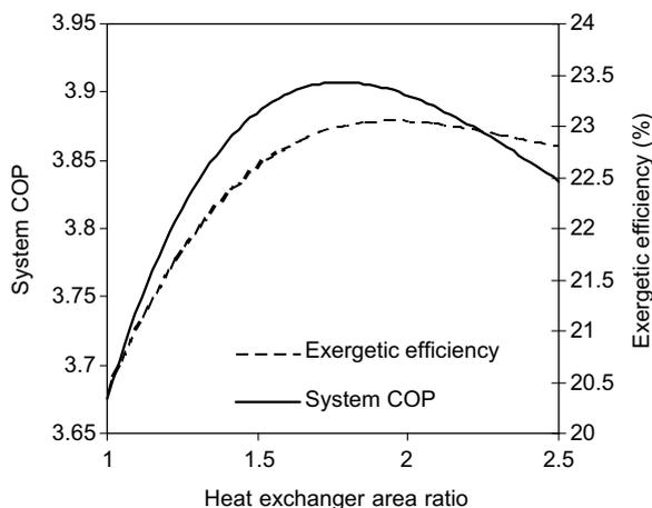
Fig. 2. System performance with varying heat exchanger area ratio.
