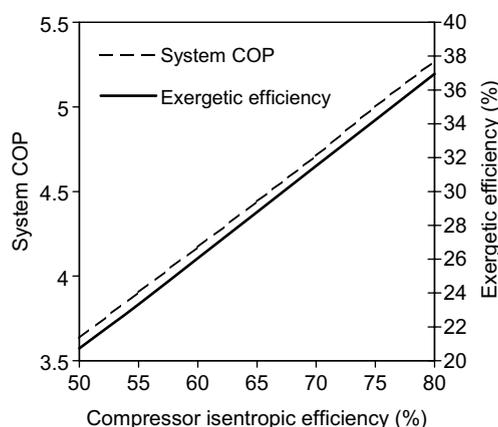
Fig. 9. System performance with varying compressor isentropic efficiency.
